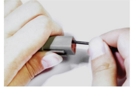
3. Push contact straight into connector until a 'click' is felt. A slight tug will confirm placement.
