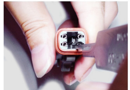
3. Use the other end side of extraction tool to expand the slot and extract contacts from connector.
