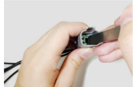
6. A 'click' will be felt when the wedge is fully installed.
