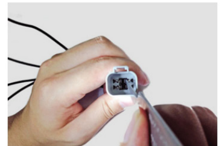
3. Use the same end of extraction tool to expand the slot and extract contacts from connector.
