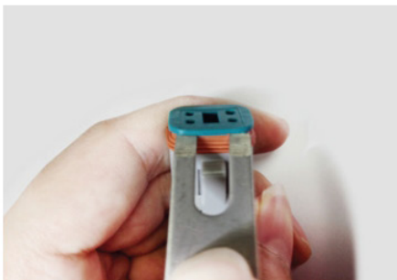
1. Insert into the lip underneath wedge by one end side of extraction tool.
