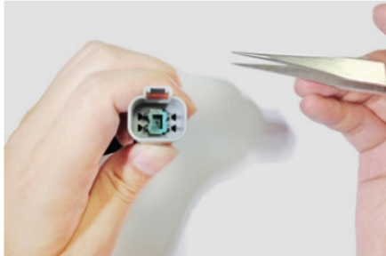
5. Put the wedge into connector with tweezers
