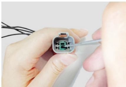
1. Hook the inside wedge by small end edge of extraction tool.
